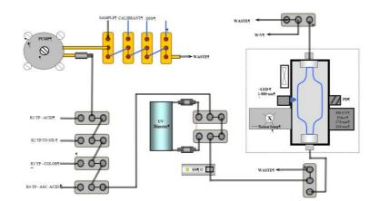
**AMMONIA** the sample reacts with salicylate in an alkaline medium pH 12, while nitroprusside acts as a catalyst. The blue color is measured at 660 nm. This method is not applicable to seawater analysis.
