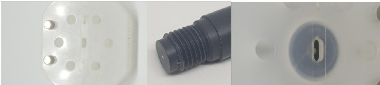
The opening is rectangular, and the flow path is cut into the piece. Note there is a gap between the bottom of the reference electrode at the path when reference electrode is installed.
