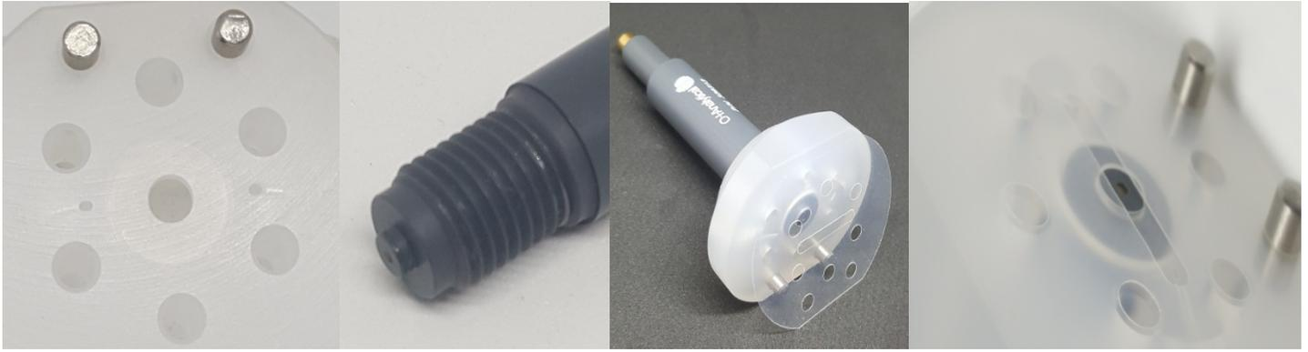
The opening is round, and a gasket is placed between the top and bottom pieces to create the flow path. Note that the bottom of the new style reference electrode has a protrusion so that it is flush and in direct contact with the fluid path when the reference electrode is installed.
