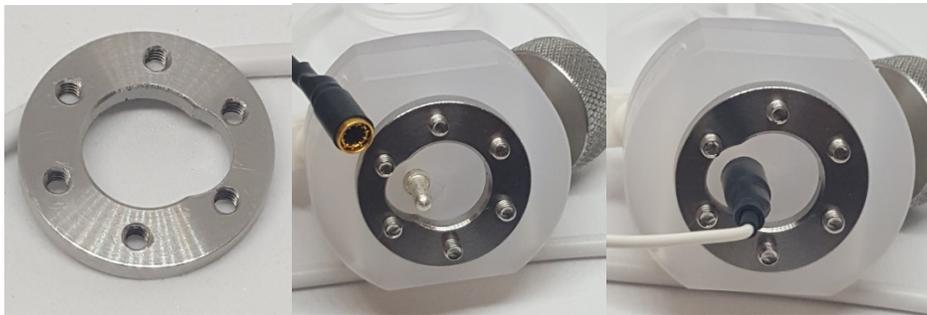
New Style Threaded Bolt Ring must be configured with the notch at the silver electrode to clear the connector.
