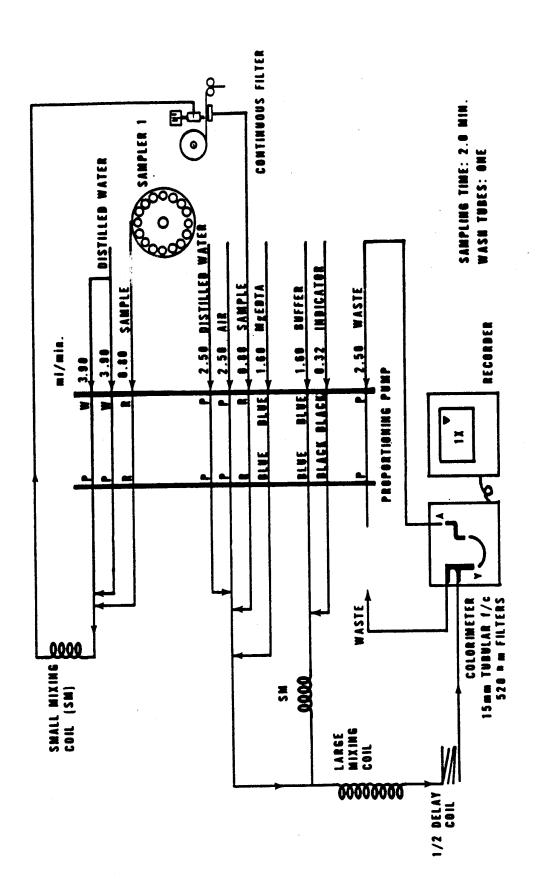
FIGURE 1. HARDNESS MANIFOLD AA-I
