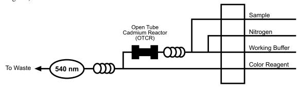
2.5 A general flow diagram of the FIA system is shown below (see Section 17.0 for a detailed flow diagram).
