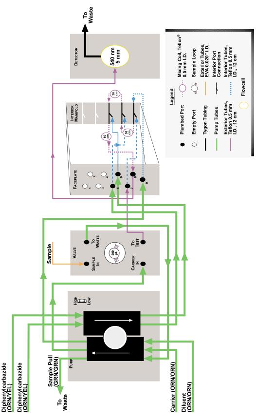
Figure 1. Detailed Flow Diagram for Hexavalent Chromium by FIA on a Flow Solution 3000, Cartridge Part #A002831
