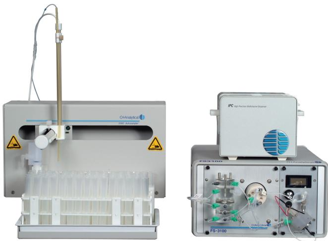
Figure 1. CNSolution™ 3100 Cyanide Analyzer
