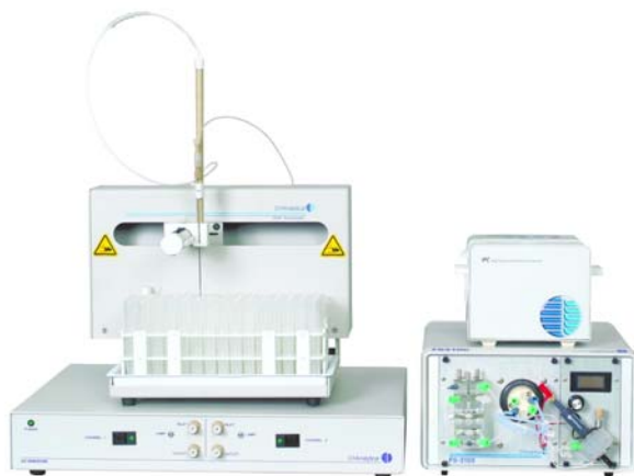
Figure 4. OI Analytical CNSolution™ 3100 Cyanide Analyzer for ASTM D 7511-09e2
