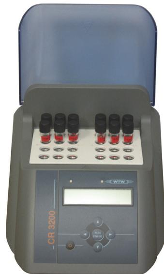
Figure 1. Thermo Reactor for Manual Digestion of Total Nitrogen and Phosphorus
